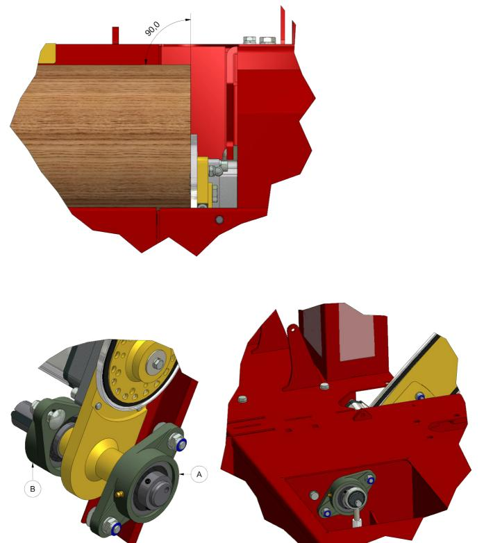
The angle of the saw bar to be adjusted by moving the bearings marked A and B as illustrated. Bearing A to be adjusted vertically and bearing B horizontally.
