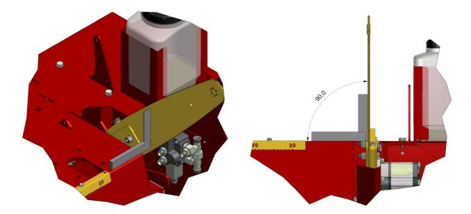
Apply a 90 degree tool in order to adjust the angle correctly for the chassis. As illustrated the bar is to be adjusted to a 90 degree angle against the feeding belt
